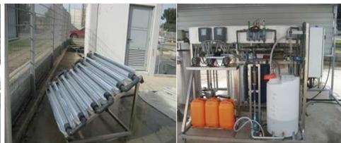
Figure 2. Compound parabolic collector (CPC) solar reactor
